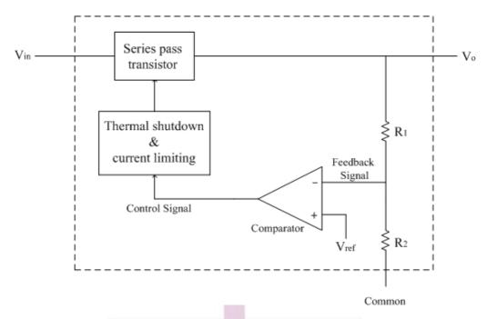
Several types of both linear (series and shunt) and switching regulators are available in integrated circuit (IC) form.
