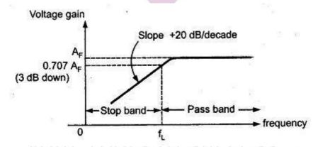
**Note:** As high pass filter is basically a low pass filter circuit with positions of R and C interchanged, the design steps and the frequency scaling method discussed earlier for low pass filter is equally applicable to the first order high pass Butterworth filter.
