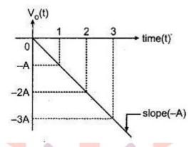
Thus output waveform is a straight line (negative going Ramp) with a slope of -A where A is magnitude of the step input. The output waveform is shown in the figure.
