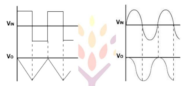
Draw the output wave form if unit step input is applied to an integrator as shown in figure.
