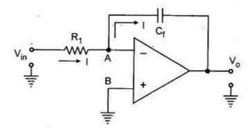
The non-inverting terminal i.e. pin - 3 of the op-amp is grounded either directly or through a resistor which is a parallel combination of input resistor Rin and feedback resistor Rf. Figure 1 shows Basic Integrator Circuit.
