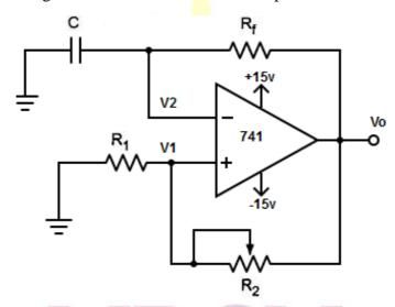
When  $V_0$  is at  $+V_{sat}$ , the feedback voltage  $V_1$  is called the upper threshold voltage  $V_{UT}$  and is given as
