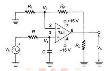
Using the voltage divider rule, the voltage across the capacitor, i.e. at the non-inverting input is
