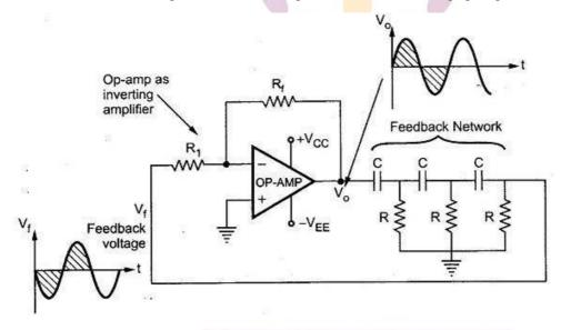
The output of amplifier is given to feedback network. The Output of feedback network drives the amplifier. The total phase shift around a loop is  $180^{\circ}$  of amplifier and  $180^{\circ}$  due to 3 RC section, thus  $360^{\circ}$ . This satisfies the required condition for positive feedback and circuit works as an oscillator.
