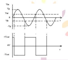
A graph of output voltage  $(V_0)$  versus input voltage  $(V_i)$  can be plotted for an invertingSchmitt Trigger Circuit Diagram, as shown in figure.
