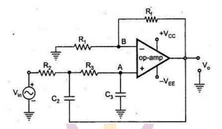
A first order filter can be converted to second order type by using an additional RC network as shown in the figure.
