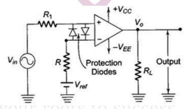
As discussed earlier, when  $V_{in}$  is greater than  $V_{ref}$  the output voltage goes to positive saturation, i.e.  $V_{out} = + V_{sat} = + V_{cc}$  and when  $V_{in}$  is less than  $V_{ref}$ , the output goes to negative saturation, i.e.  $V_{out} = -V_{sat} = -V_{EE}$ .
