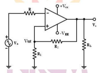
The input voltage  $V_{in}$  triggers (changes the state of) output  $V_{out}$  every time it exceeds certain voltage levels called upper threshold  $V_{ut}$  and lower threshold voltage  $V_{lt}$  as shown in figure.
