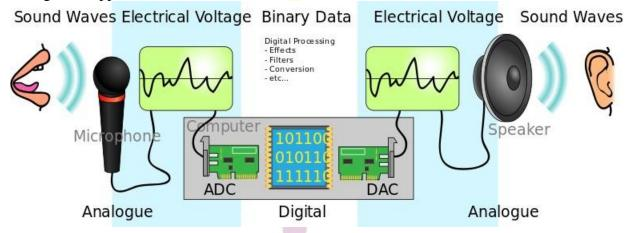
Fig.: Illustration of ADC and DAC
