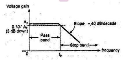
At the cut off frequency  $f_H$ , the gain is 0,707  $A_f$  i,e. 3 dB down from its 0 Hz level. After,  $f_H$  (  $f > f_H$  ) the gain rolls off at a frequency rate of 40 dB/decade,. Hence, the slope of the 'response after,  $f_H$  is -40 dB/decade.
