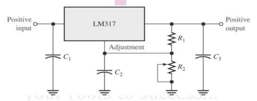
The three terminals are V<sub>in</sub>, V<sub>out</sub>, and Adjustment(adj).
