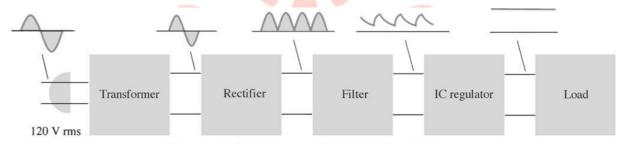
Block diagram of a power supply which uses IC regulator is as shown in figure
