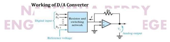
Fig.: Block diagram of DAC
