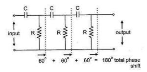
The network is also called the **ladder network.** All the resistance values and all the capacitance values are same, so that for a particular frequency, each section of R and C produces a same phase shift of 60°.
