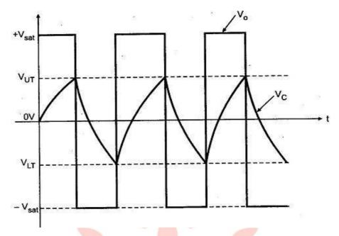
The current I discharges capacitor to 0 V and recharges capacitor to  $V_{LT}$ . When  $V_c$  becomes slightly more negative than the feedback voltage  $V_{LT}$ , the non inverting (+) input is higher than inverting (-) input. This switches the output voltage from -Vsat to
