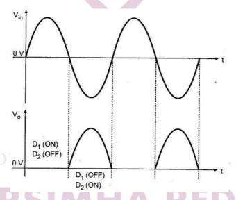
Non inverting Half Wave Rectifier which rectifies negative half cycle:
