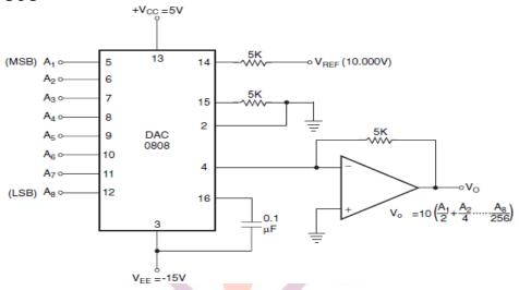
Fig.: DAC 0808 wired as a voltage-output D/A converter
