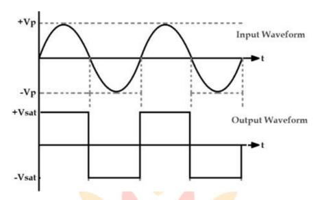
If the op-amp non-inverting input is grounded and the signal is applied to the inverting input then output is negative when the input is above ground, and vice versa. Because of the waveform inversion, this circuit is often termed an **inverter**
